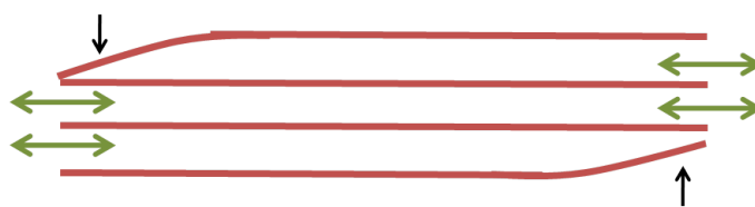
Figure 8.8: The desorption of the interlayer water molecules can be disturbed by the collapse of the crystal layers that create the interlayer pore. The black arrows represent such collapses at different places of the model that would reduce the water exchange and the green double arrows represent an easier exchange where there is no layer collapse.
