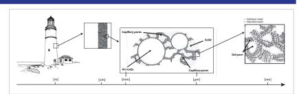
For the past 20 years, <sup>1</sup>H Nuclear Magnetic Resonance (NMR) has been used in order to study the water in cementitious materials. With a resolution of one molecule, the water held in the C-S-H nanostructure can be measured and studied. The aim of this project is to use this new tool to better describe the porosity of cement-based material. The NMR results will act as a basis of comparison with the other «classical» characterisation methods.
