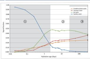
The diagram shows the evolution of the different water signal fractions over the time. There are 3 main stages
