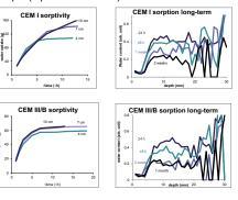
Half of the water disappears from the profiles in 2 weeks on both CEM I and CEM III/B. CEM III/B was measured up to a month and there was no change in weight or water profile after 2 weeks. The samples were minimum 6 month old.
