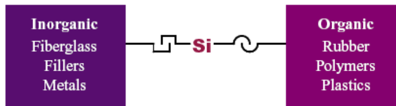
Figure 2-12. The silane coupling mechanism (reproduced from [48])
