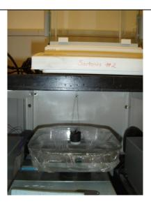
Fig. XV.2: Set up for capillary suction test.
