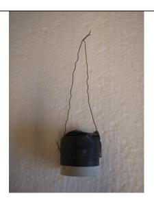
Fig. XV.1: Sample with plastic around to prevent evaporation.
