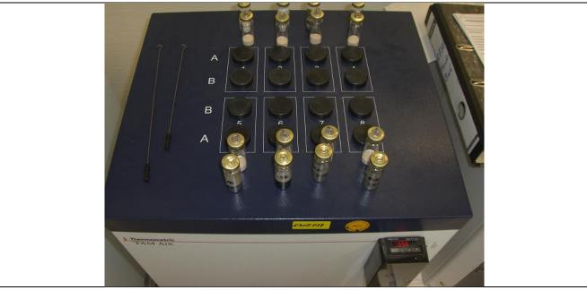
Fig. XIV.3:Thermal calorimeter and the ampoules
