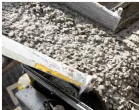
approximately 70-80% of the mixture and cement and water make up the rest. Aggregates are usually inert coarse materials like gravel, crushed stone, sand or recycled concrete. The type of aggregate selected depends on the local availability and the application of the concrete.
